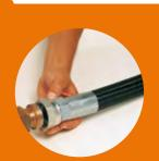
Position the fitting near the male coupling.
