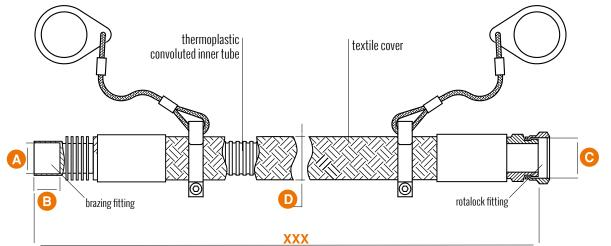
INFINITY HOSE with Rotalock fitting and brazing metric fitting (with safety clamp)
