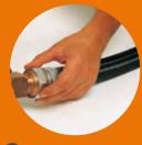
2 Screw the fitting thread onto the male fitting, clockwise by hand for the first few turns.
