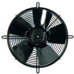
Stamped steel blades (type 28 °, 30 °, 32 °) Diameters: 250-350 mm
